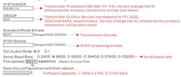
Receiver module: (Since the receiver has four decoders, there are four corresponding IP addresses need to be configured)
