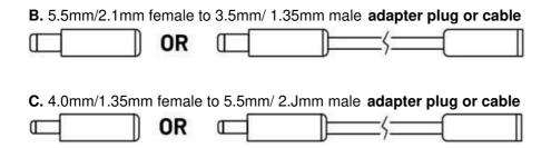
Note: Either Adapter Plug or Adapter Cable would be included in the package. Their function is same.
