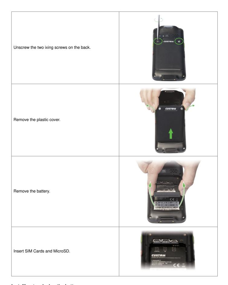
Installing / replacing the battery
