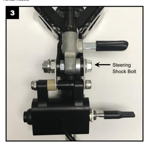
4. Determine the hanging mounting position of the SXS Turn Signal Switch and tighten the Steering Shock Bolt to the OEM torque spec.
