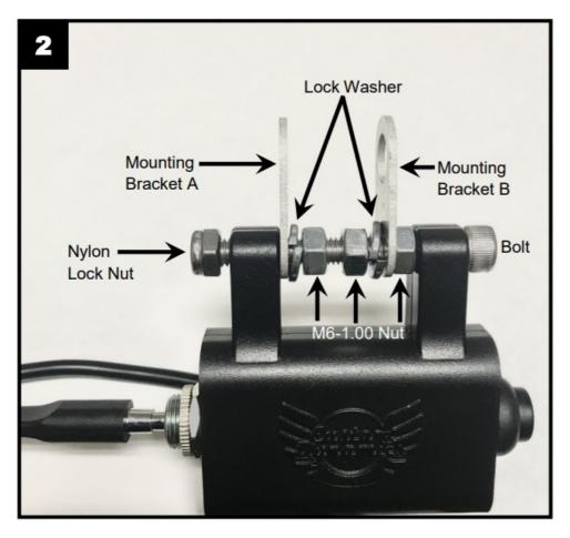
3. Using the OEM top tilt steering shock bolt mount the SXS Turn Signal Switch along with the tilt steering shock to the steering pivot tube. Refer to Photo #3 for Kawasaki models. Refer to Photo #4 for Polaris, CanAm, and Honda models.
