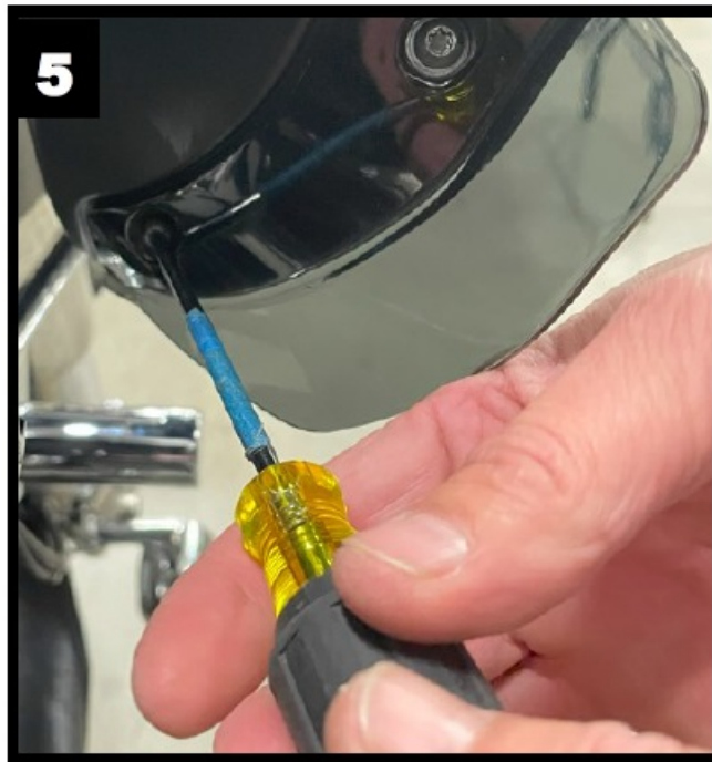
5. Remove both left and right lower T-25 torx bolts from the bottom of each fairing chin spoiler. Shown in Figure 5.
