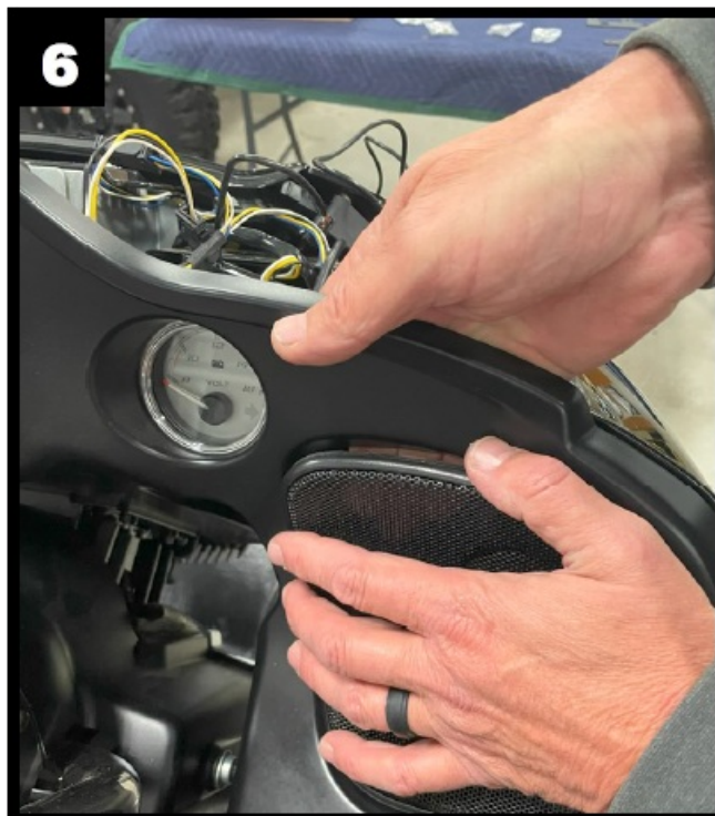
6. The speaker grills are held in by clips. Remove both left and right speaker grills on the inner fairing by pushing outwards from the inside of the speaker grill. Shown in Figure 6.
