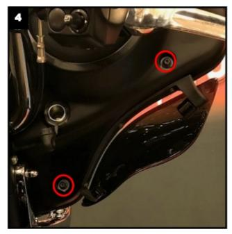
4. Remove the 3 top T27 Torx Bolts from the outer fairing as shown in Picture 3. Remove the windshield and store it in a safe place for reinstallation later.
