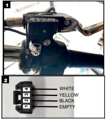
8. Pins should snap in place and not pull back out of connector when installed correctly.
