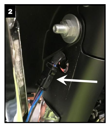
Unplug the connector by pushing in on the tab located on the male side of the connection as shown in Picture
