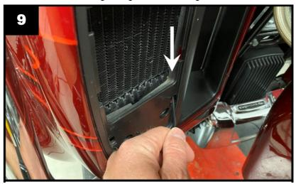
20. Gently pull back on the inside of the rear Lower Fairing cover and pull the Lower Fairing wiring harness through the lower Fairing as shown in Photos 10 and 11.
