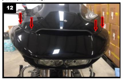
2. Once the windshield fasteners and windshield are removed, you will need to remove the vent. The vent is secured to the fairing by clips. Position yourself in the front of the motorcycle and lift straight up on the vent to release. Refer to Photo 13.
