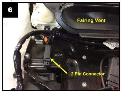
14. Remove the Black connector plug from the 2 pin fairing Power and Accessory connector on the motorcycle by pushing the center tab in and pulling the plug out. Save the plug for reinstallation later. See Picture 7.
