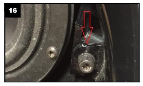
7. Locate and remove the lower T-25 screw on each side of the inner fairing. Refer to Photo 17.
