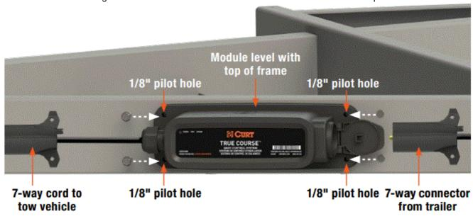
**Note**: Before positioning the module for marks, make sure there is adequate length on the attached front 7-way cord to connect to the tow vehicle.
