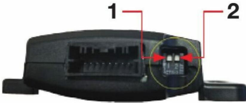
There are two small switches located at the front of the unit, next to the port on the module. Once accessed, the switch positions can be changed using a small pointed tool.
