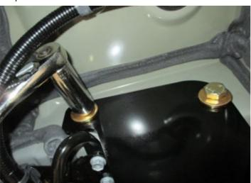
**Step 5**Raise the exhaust back into position and reinstall the isolators if lowered in step 2.
