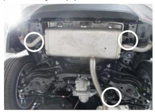
**Step 3**Raise the hitch into position and install the four hex bolts (#1) and four conical-toothed washers (#2).
