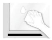
1. Locate Background LED light mounting location and clean of any dirt, algae or debris.
