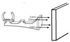
4. Attach stand mounts to back of stand using 4 small wood screws. (NOTE: 3M adhesive tape is also included for installation, Skip to Step 6 below.)
