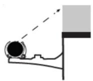
5. Insert Background LED light into swivel clips and swivel LEDs to illuminate background film.
