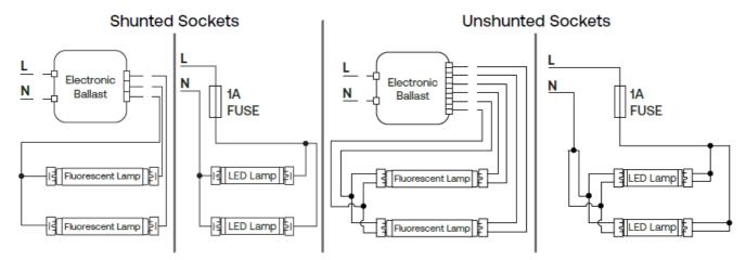
Type B Tube Misapplication In-Line Fuse Kit
