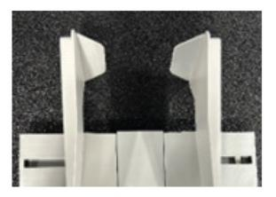
5. Place the hopper support in the machine as shown and fastened with your hands placing the washers first and then the wing nuts.
