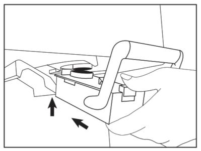
4. Slide the condiment chute into the space provided under the condiment containers. Be sure to slide it all the way in until it stops.
