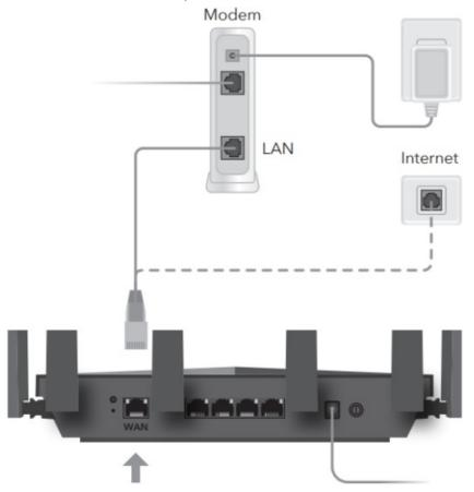
3. Connect the router via A or B method.
