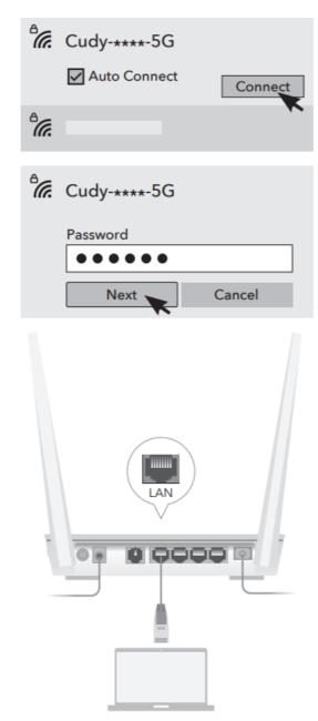
5. Open a browser on a device that is connected to the router and follow the picture to change the Wi-Fi password.
