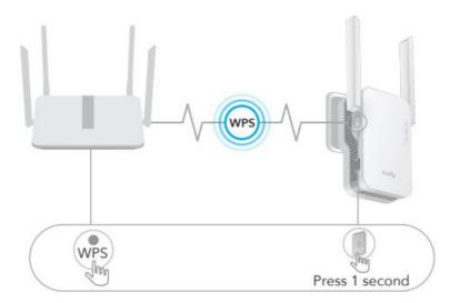
3. Then the LED will start to flash wait until the LED and LED turn solid on, which means the extender connects to your existing host WiFi network.
