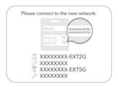
Note: Please check the information on the screen and confirm that the password is the same as the wifi password of the router. Otherwise, the extender will not be able to connect to the router WiFi.
