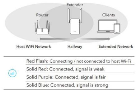
5. Connect your device to the extender using the extended SSID and WiFi password that you've set during the configuration. The default WiFi password is the same as your host WiFi network (router WiFi).
