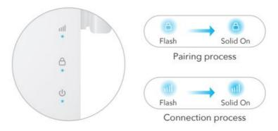
If the LED does not turn solid on after 2 minutes, try step 2 again. If still not work, try Method Two: Using Web Browser, or contact our support team <a href="mailto:support@cudy.com">support@cudy.com</a>.
