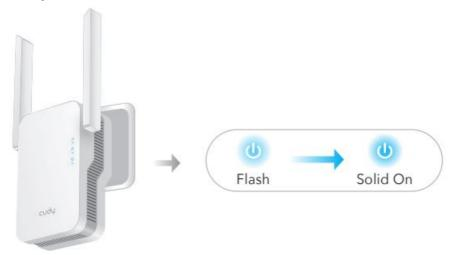
2. Press the WPS button on your router, and then press the WPS button on the extender within 2 minutes.
