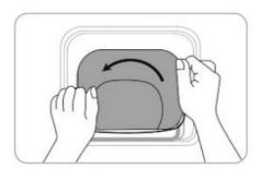
2. Place the bread pan back into the bread maker. Ensure the pan is firmly locked into place by turning it clockwise. Then, close the lid.
