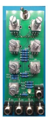
When everything is in place, put the front panel on top, so all controls go into each corresponding hole of the panel. Make sure everything fits well. Fit all nuts to the Potentiometers and Jacks. Be careful when turning the boards around, so that the components stay in place. Then solder everything.
