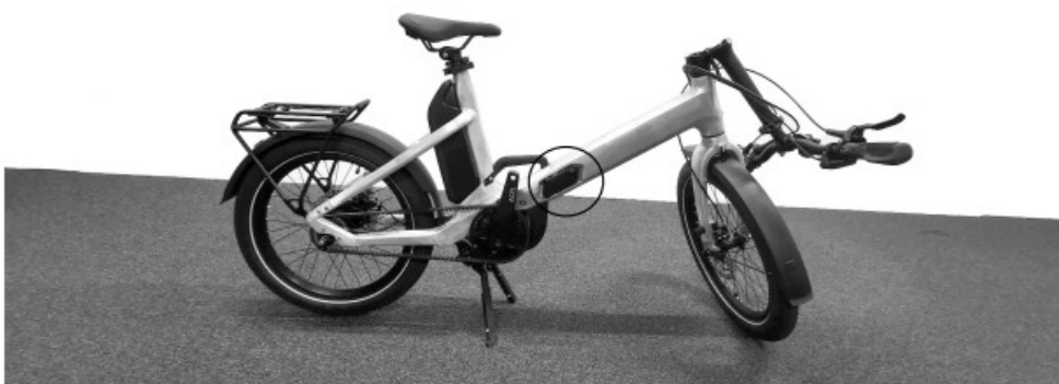
Fig. 4: Unlock folding mechanism
