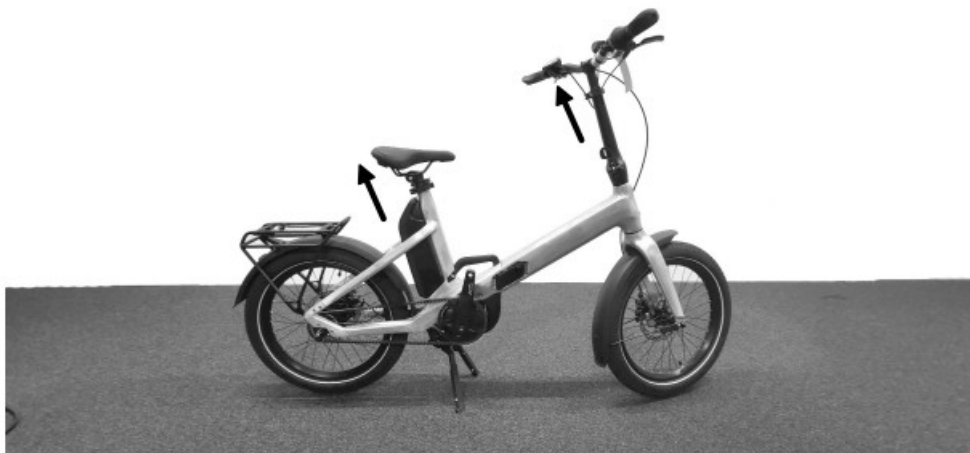
Fig. 15: Adjust stem and saddle height
