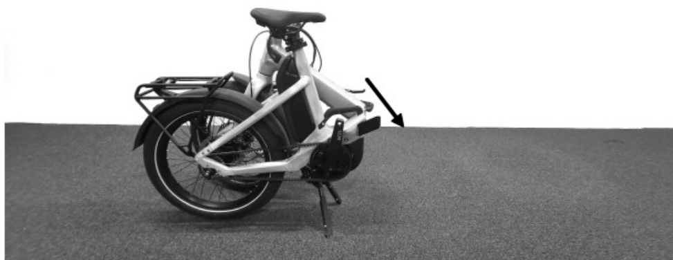
Fig. 11: Swing front frame (open)
