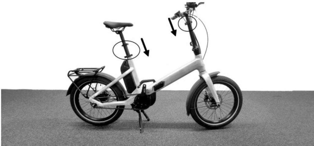
Fig. 2: Draw in Seatpost + stem
