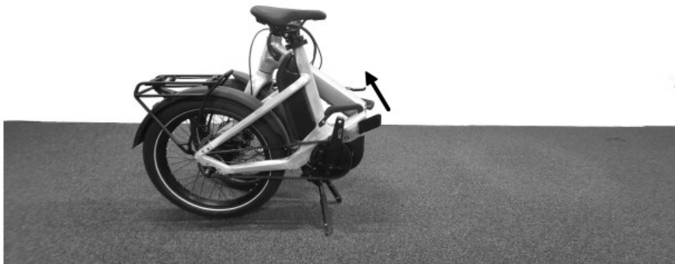
Fig. 6: Swing front frame part (close)
