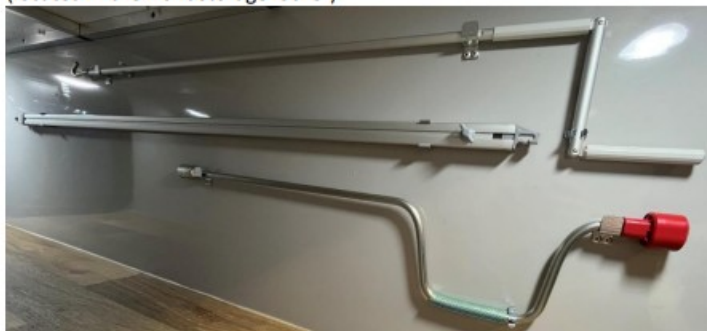
Fiamma Awning Winder, Fiamma Tension Rafter, and AL-KO Winder Handle (Top to Bottom) (located in the front storage locker)
