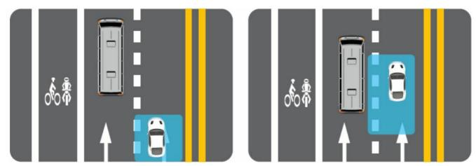
• If the blind spot indicator on the left A-pillar lights up or flashes, it indicates that there is a vehicle entering the left side of your vehicle or a vehicle approaching from the rear left side at high speed. Please slow down and check your surroundings before safely continuing.
