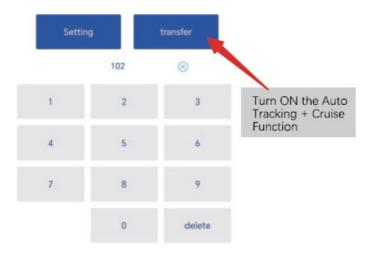
Turn OFF Auto Tracking+ Cruise Function: If you need to turn off auto tracking, enter 103 and click "transfer". (Note: After opening the tracking cruise function, you must call this command to close this cruise.)
