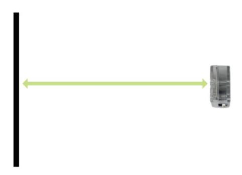
For best results, keep the detection surface and the CANrange parallel.
