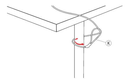
**4B.** Attach cable lock head (K) onto the enclosure k-slot location (A) then insert provided key (J) and tum it clockwise. Remove key to lock and secure.
