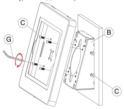
3A. Align enclosure holes (A) to VESA wedge holes (B) then tun in screws (C) using provided tool (G)
