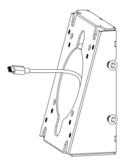
**2B**. Align VESA holes of tablet security enclosure (A) to that of the wedge (B). Rotate in (4) screws (C) from the front using provided tool (G) until securely fastened.
