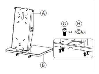
1A. Align base (B) to body (A) as shown. From below, rotate in (4) screws (G) and washers (H) as shown using provided tool (D) until securely tightened.
