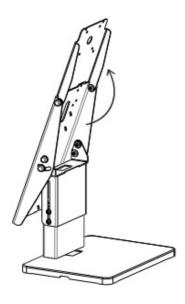
3A. Identify the top VESA plate, Tilt it down for a 2-direction setup or keep it up for a 1-direction setup as required.
