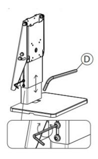
2A. Loosen the side bolt using provided tool (D) to raise or lower to height to your preference. Rotate opposite direction to securely tighten and set your height.
