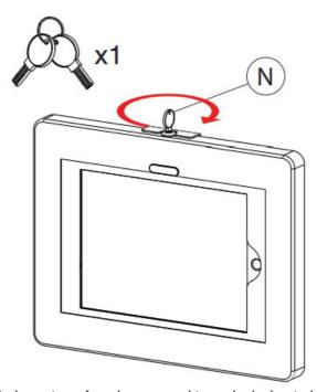
7B. Insert the key (N) in the keyhole on top of enclosure, and turn clockwise to lock the enclosure in place.
