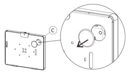
6A. When installing device into enclosure (C), identify where the camera is. Then simply remove and pop out the cover prior to mounting or setting up tablet to properly expose camera.
