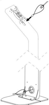
2B. When the cable reaches the bottom of the stand, pull through the hole at the stand back and remove the weighted pendant as shown.
