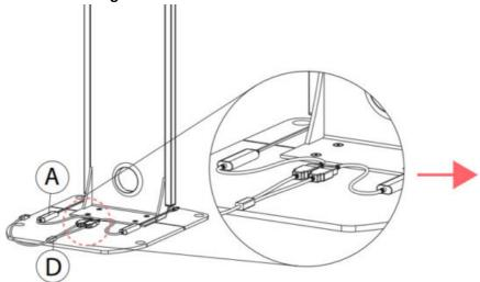
10A. Take the cables attached to the LED (A) and attach them to the bottom half power cable (B) via USB connection.
