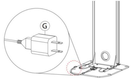
11B. Attach the power adapter (D) to the end of the cable as illustrated. Then plug into power source as needed.
