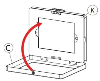
7A. Once the tablet device is set up, close the front lid of the enclosure (C).
