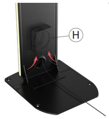
10B. Route all the cables into the cable storage component (E) as illustrated.
