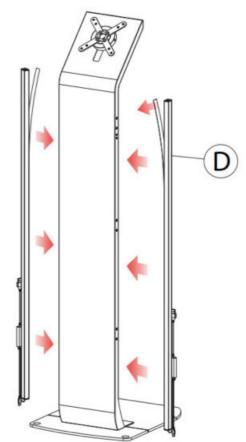
1A. Peel off the 3M adhesive sticker on the back of the LED light bar (D) as illustrated. Attach the LED bar onto the edge of the CTA floor stand with the wire end on the bottom side. Repeat same steps for the LED bar on the other side of the floor stand.
