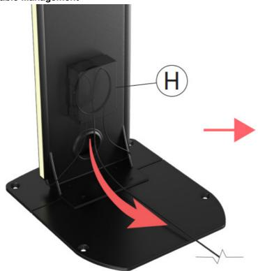
11A. Route the power cable out the bottom of the cable storage (H)
