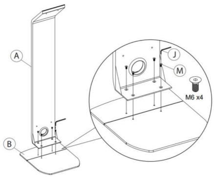
1A. Allign the holes on the sntad (A) with holes on the base (B) and turn in screws (M) with provided allen tool (J) until securely tightened. Shown above.
