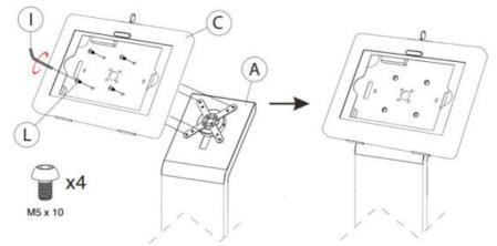
3A. Align enclosure (C) VESA holes to VESA plate holes in stand (A) and from the front of enclosure turn in screws (L) into the threaded VESA holes with provided allen tool (I) until securely thigtened. Shown above.
