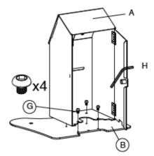
• 1A. Connect base (B) with body (A). Take the body (A) and align the mounting holes. Rotate in (4) screws(G) with provided Allen key (H) until securely tightened.
