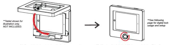
6A. Once tablet is inserted, close the front cover securely.
