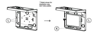
• 5A. With the enclosure open, insert the tablet into the foam adapters (L). Make sure the adhesives have been placed ahead of time or the tablet will fall out. Plug your tablet into any cables/wires you have routed to the enclosure. After the tablet is secure, close the top and lock it into place.
