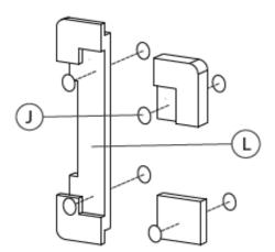
• 4A. Identify the double-sided adhesives (J). Peel away the backing on both sides. Adhesive four of them behind the foam pieces (L) as illustrated. They are to adhere the foam to the enclosure. Peel away the back on the next four and place them on top of the foam pieces as illustrated. These are to attach the foam to the tablets and ensure security.
