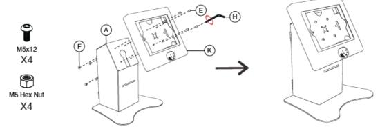
3A. Align the VESA holes of the enclosure (K) to the VESA holes of the kiosk body (A). Rotate in screws
