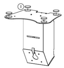
• 2A. Flip over the now combined base section. Find the base pads (component I) and peel off the sticker to expose the adhesive. Place the foam pads (adhesive face down on base) at the corners and give it a firm press for a few seconds until it's securely attached.
