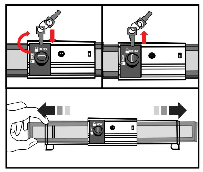
2. Insert key and lock the holder, take out the key, then insert your device corner first. Slide the arm back in until it is tightly gripping your tablet by the corners.
