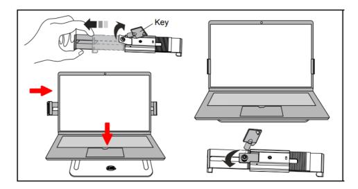
• The higle of the holder allows you to adjust your Laptop screen angle.Loosen and tighten the screw of the hingle with Allen Key to adjust the angle of the holder.
