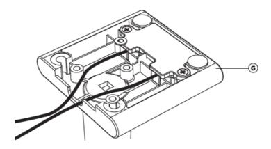
1B. Prior to beginning the grommet or clamp installation – press the USB cables into the groove as shown to properly setup.
