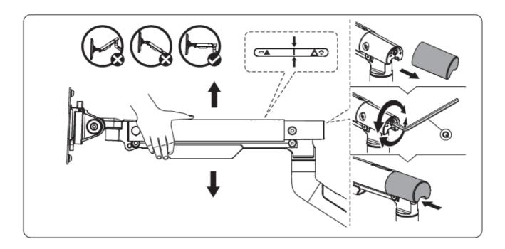
To properly balance the arms with monitors mounted, adjust the spring tension using the provided allen key. Position it in the horizontal position and firmly hold the arm as shown. Tight the screw to fix it in the horizontal position.
