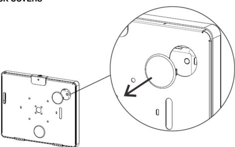
Remove or retain back covers as needed. Typically, where the camera is, you will remove the cover. Simply pop out cover with fingers prior to inserting tablet into enclosure.
