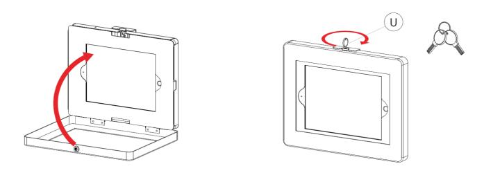
Once the tablet device is set up, close the front lid of the enclosure.
