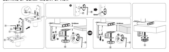
Align L-shape component(F) with base of clamp mount as shown above. Rotate in screws (K) through using provided tool (P) until securely tighten. Afterwards peel off sticker back of padding (N) and place firmly on the screws (K).
