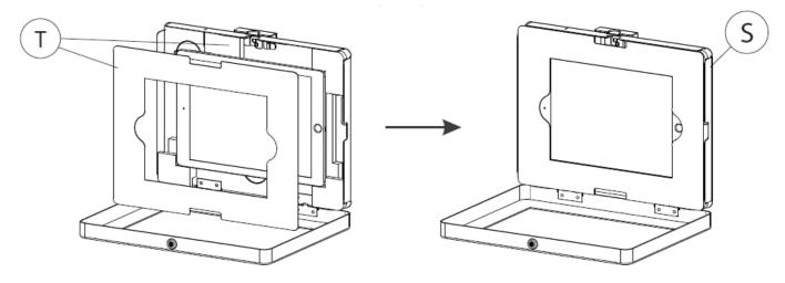
Lay-in correct masking insert from the bundle (T) as
