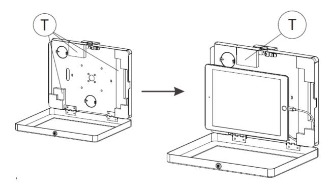
Find the appropriate size foam padding (T) for the tablet you wish to use. Make sure the device is compatible for the enclosure. If having a power/data cord attached to the tablet, slide it through the back of the foam as shown and out the opening in the back.
