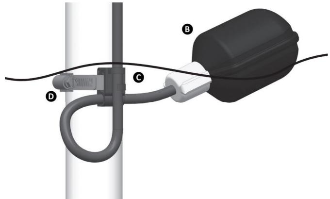
3. Remove screw from front of lower cover. Lift bottom of lower cover out slightly. Slide lower cover down until it is clear of the upper cover and remove. Determine "conduit-in" location on alarm. See bottom of enclosure for cord placement indicator marks. Drill holes for conduit entry.
