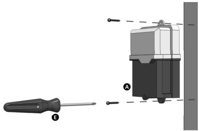
2. Install float switch at desired activation level.
