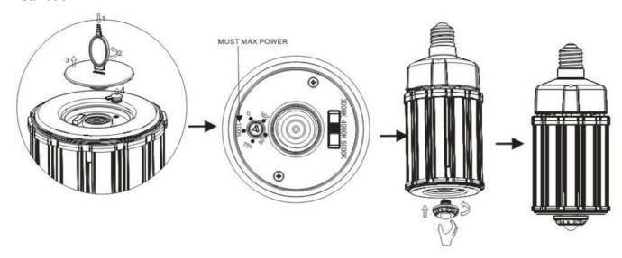
It could be easily installed using a straight screwdriver. Use a flat-blade screwdriver to unscrew the plug and remove the plug. And then. Choose a motion sensor to install and tighten.
