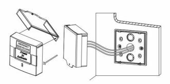
Put the protection cover onto the front case and connect the wire correctly.
