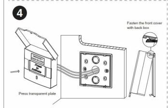
Fasten the front case on the back box. (Remark: before fasten the front case, you could test the function first. You could press the pressing plate and the buzzer will sound or silent and LED will change the color. LED will keep lighting or flashing base on your jump cap position)
