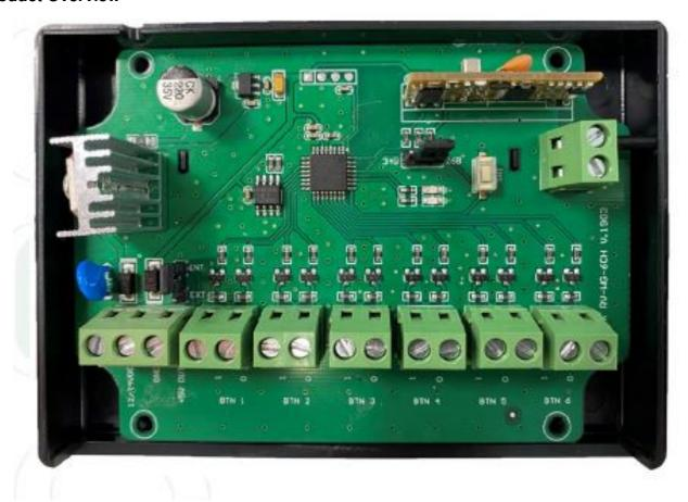
The CS Technologies 6 channel Wiegand receiver is a long-range, high-security RF receiver which employs KEELOQ® code hopping encryption technology. It provides 6 output channels of 26-bit Wiegand protocol and connects to the access controller in the same way as 6 separate card readers would. 2 and 4 button CS RF transmitters are available.
