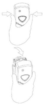
**Note:** DO NOT use a screw driver or other implement to remove cover. Incorrect removal of cover may damage the LED and void the warranty.
