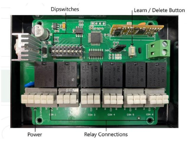
For best performance the receiver should not be installed on or next to a metallic surface. If the receiving distance is poor or you get interference from other devices you may improve this by relocating the receiver to another location.
