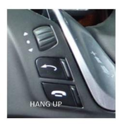
camera ANG UP button on the steering wheel control for 3 seconds to manualy activate or deactivate the front camera.
