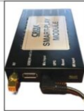
12. Plug in the microphone cable to the Smart-Play module. Optional plug in original smartphone cable to USB Ext. cable for wired connectivity
