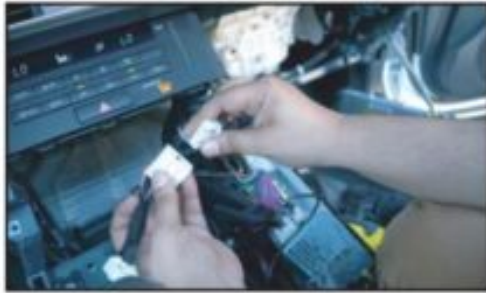
Plug in the AUX-IN t-harness to the factory radio aux connector.
