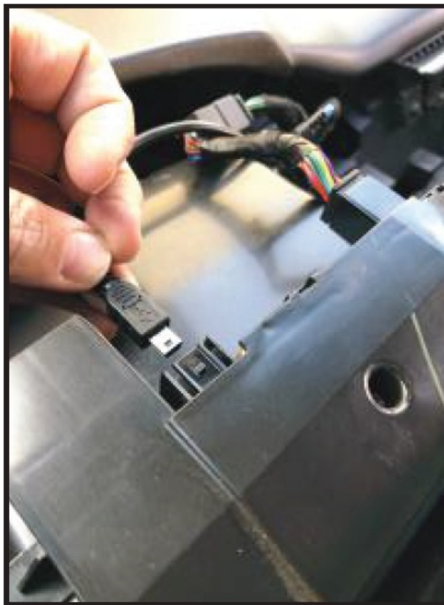
ACPGM-80N LVDS video cable plugs behind radio
