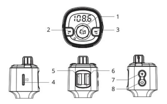
Answer / Hang-up / Reject / Redial a call: Press the button to Answer / Hang up a call. Long press the button to Reject a call. Double Press the button to redial the last dialed number.
