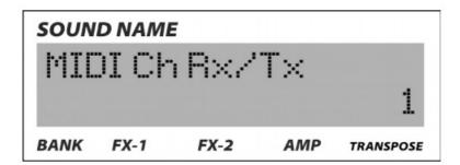
Seventeen has a dedicated button in the panel for MIDI LOCAL OFF: when this function is engaged, the instrument does not produce sound anymore and it will start sending MIDI messages on a MIDI channel that you can choose between 1 and 16.
