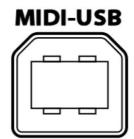
An additional Type-B USB 2.0 port is present at the back side of the Mojo that provides Class-compliant USB-MIDI IN/OUT connection to your computer. Use this port to connect the Mojo to your computer software. No drivers are needed for Windows, OS X and Linux.
