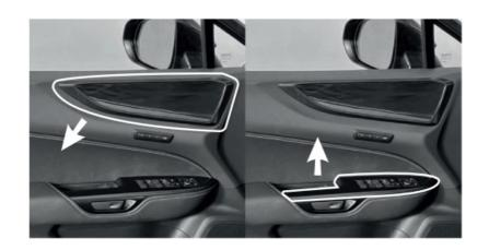
In most cases the screws used are Phillips type, use a tool bit PH2 size. Unscrew them and store the screws in a safe place, for later use when reinstalling the door panel.
