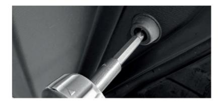
To remove the door panel, all clips need to be released. Loosen the door panel by inserting the pry tool between the panel and the door. Pry the door panel gently, but firm, outward to release the clips.
