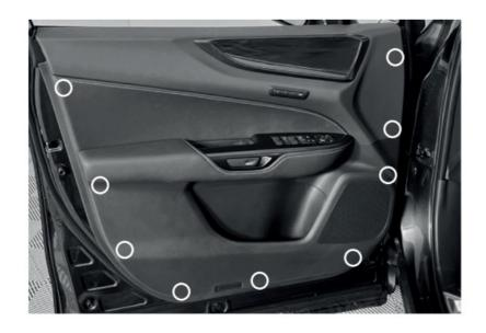
Usually the clips/screws are placed by the white marks. This could vary depending on the vehicle.
