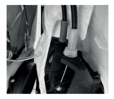
Disconnect electrical connections for the door lights.
