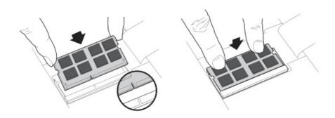
• Firmly push the SODIMM in at a 45-degree angle, and then push down until clips snap into place.
