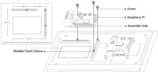
Adjust the sliding retention post to match the Raspberry Pi and attach the screws to the CrowVision sliding retention post through the Raspberry Pi's fixing holes.
