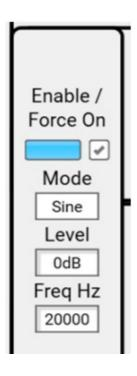
There is one signal generator per amplifier. It injects its signal on the input side of the DSP chain and passes through the DSP.
