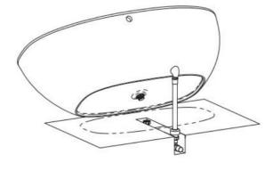
Tub thicknesses range from 9/16" to 3/4". Please check and use the appropriate connecting screw from the table below.
