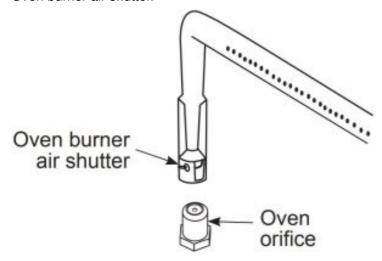
**NOTICE:** This product cannot be converted to propane (LP) by adjusting the oven orifices. The orifices must be replaced for propane (LP).
