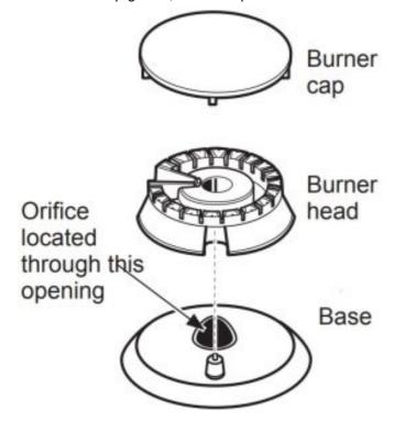
2. Using a 7 mm or 9/32" nut driver, remove the top burner orifices. These may be accessed through the burner opening in the base.
