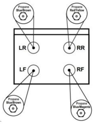
4. Install the propane (LP) orifices in their precise locations.
